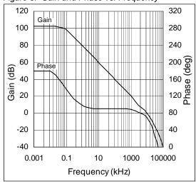
Figure 4. Gain and Phase vs. Frequency, CLOAD = 100pF
