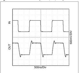
Figure 20. Transient Response, 2V, 100pF load
