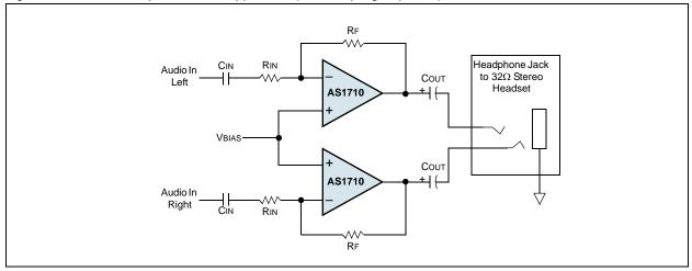
In Figure 22, CIN and RIN form a high-pass filter that removes the DC bias from the incoming signal. The -3dB point of the high-pass filter is given by:
