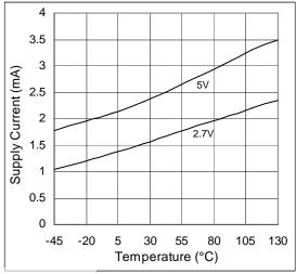
Figure 8. Shutdown Current vs. Temperature
