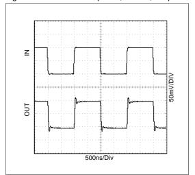
Figure 18. Transient Response, 1V, 100pF load
