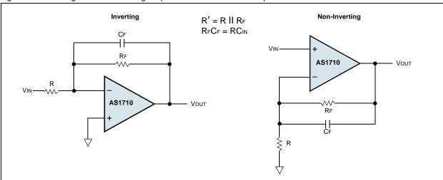
The pole frequency is 10MHz when R' =  $2k\Omega$ . To maximize stability, R' <<  $2k\Omega$  is recommended.
