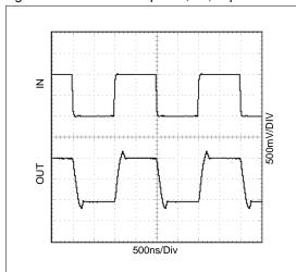
Figure 19. Transient Response, 2V, 10pF load
