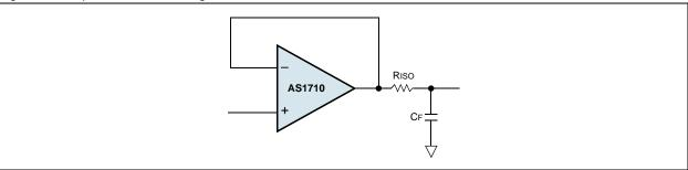
**Note:** Resistor Riso improves the circuit's phase margin by isolating the load capacitor from the AS1710/AS1712 output.
