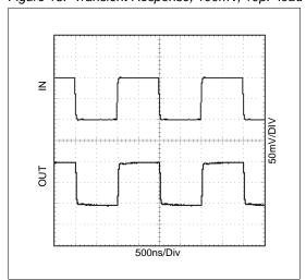
Figure 17. Transient Response, 1V, 10pF load
