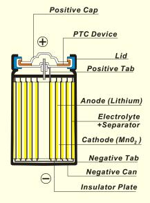
Fig.3 Spiral construction Schematic construction of a Li/MnO₂cylindrical cell (CR 123A)
