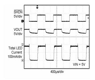
Figure 1. Switching Waveform with 1kHz PWM on SHDN
