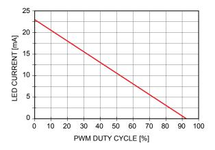
Figure 3. Filtered PWM Dimming [0V to 2.5V]
