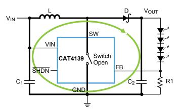
Figure 5. Open-switch Current Loop
