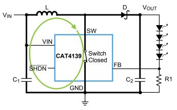
Figure 4. Closed-switch Current Loop
