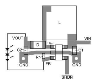
Figure 6. Recommended PCB Layout
