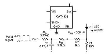
Figure 2. Circuit for Filtered PWM Signal
