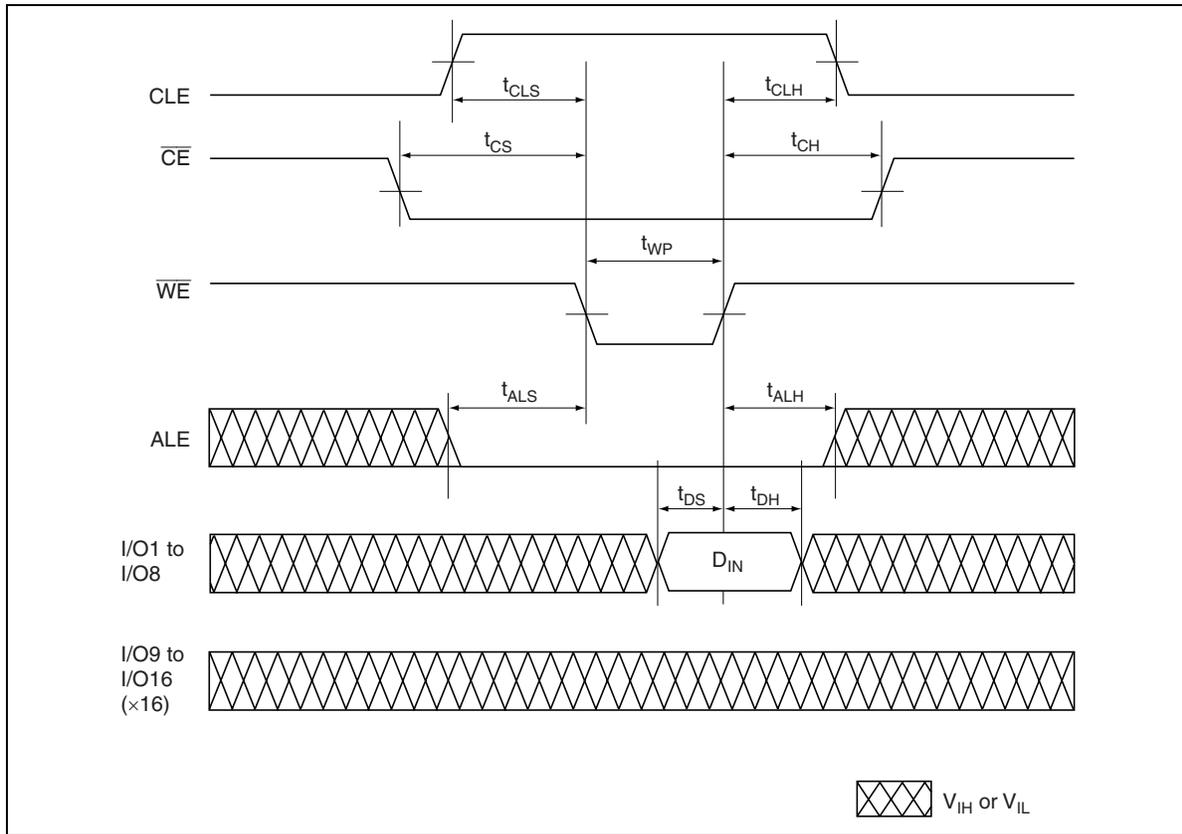
Command input cycle after data output cycle
