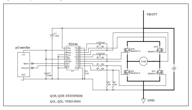
Figure 3 : Autoprotected H-bridge
