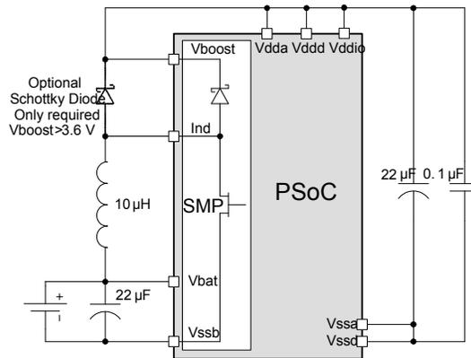
The switching frequency can be set to 100 kHz, 400 kHz, 2 MHz, or 32 kHz to optimize efficiency and component cost. The 100 kHz, 400 kHz, and 2 MHz switching frequencies are generated using oscillators internal to the boost converter block. When the 32-kHz switching frequency is selected, the clock is derived from a 32 kHz external crystal oscillator. The 32-kHz external clock is primarily intended for boost standby mode.
