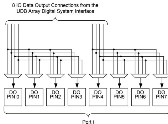
There are four more DSI connections to a given I/O port to implement dynamic output enable control of pins. This connectivity gives a range of options, from fully ganged 8-bits controlled by one signal, to up to four individually controlled pins. The output enable signal is useful for creating tri-state bidirectional pins and buses.
