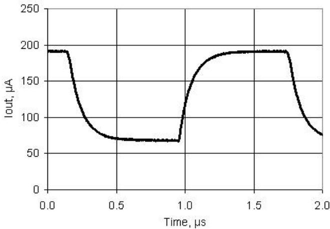
Figure 11-37. IDAC Glitch Response, Codes 0x7F - 0x80, 255  $\mu$ A Mode, Source Mode, Fast Mode, V<sub>DDA</sub> = 5 V
