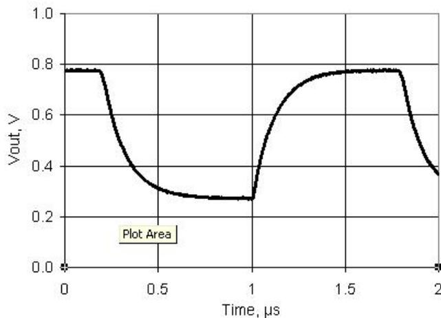
Figure 11-48. VDAC Glitch Response, Codes 0x7F - 0x80, 1 V Mode, Fast Mode, V<sub>dda</sub> = 5 V
