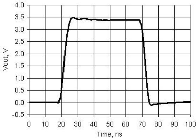
**Figure 11-16. GPIO Output Rise and Fall Times, Slow Strong Mode, V<sub>DDIO</sub> = 3.3 V, 25 pF Load**
