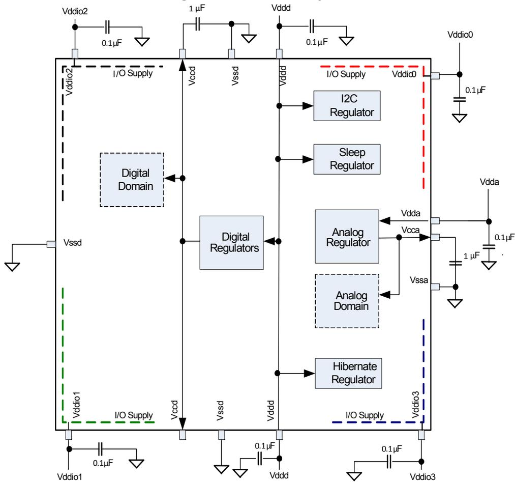
**Note** The two Vcccd pins must be connected together with as short a trace as possible. A trace under the device is recommended, as shown in Figure 2-6.
