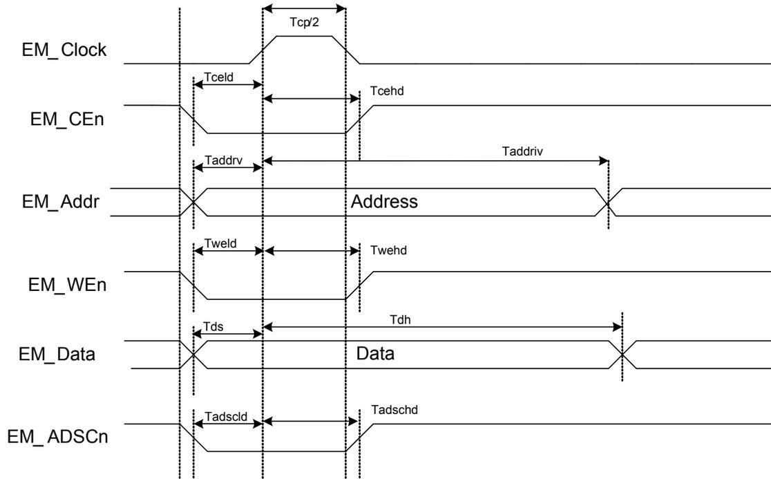
Table 11-55. Synchronous Write Cycle Specifications
