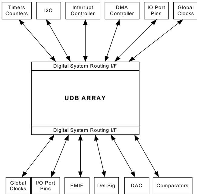
Interrupt and DMA routing is very flexible in the CY8C32 programmable architecture. In addition to the numerous fixed function peripherals that can generate interrupt requests, any data signal in the UDB array routing can also be used to generate a request. A single peripheral may generate multiple independent interrupt requests simplifying system and firmware design. Figure 7-14 shows the structure of the IDMUX (Interrupt/DMA Multiplexer).
