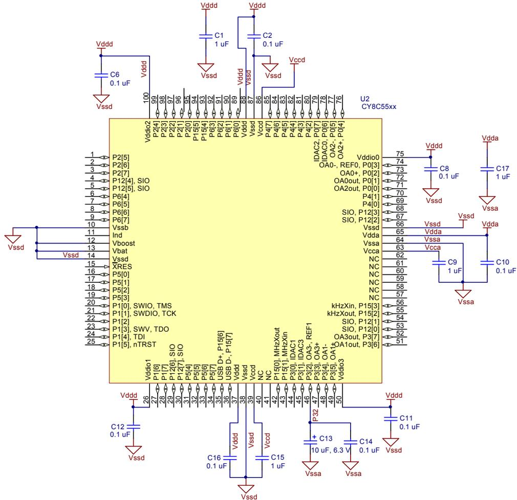
**Note** The two Vcc pins must be connected together with as short a trace as possible. A trace under the device is recommended, as shown in Figure 2-6 on page 10.
