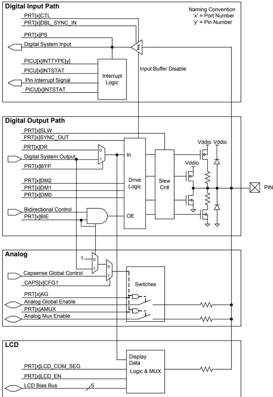
Figure 6-9. SIO Input/Output Block Diagram
