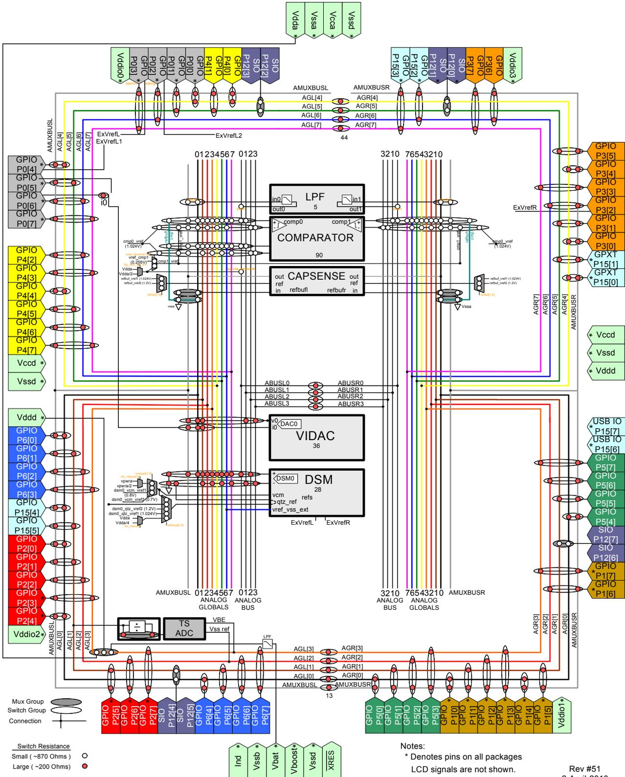
Analog local buses (abus) are routing resources located within the analog subsystem and are used to route signals between different analog blocks. There are eight abus routes in CY8C32, four in the left half (abusl [0:3]) and four in the right half (abusr [0:3]) as shown in Figure 8-2. Using the abus saves the analog globals and analog mux buses from being used for interconnecting the analog blocks.
