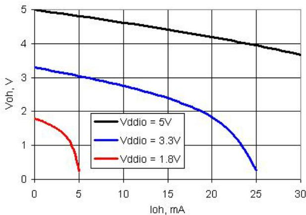
**Figure 11-14. GPIO Output Low Voltage and Current**
