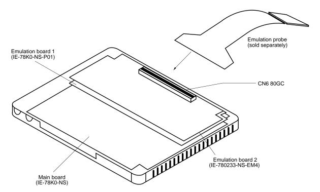
Figure 3-1. Connection of Emulation Probe
