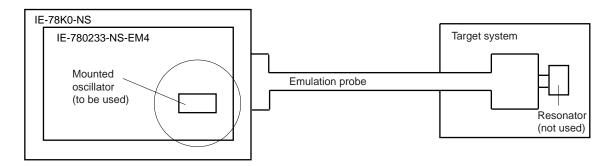
**Remark** The clock that is supplied by the IE-780233-NS-EM4's oscillator (encircled in the figure) is used.
