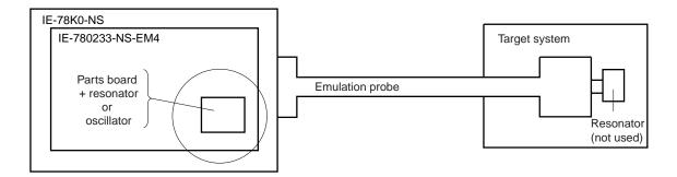
**Remark** The clock that is supplied by the IE-780233-NS-EM4's resonator or oscillator (encircled in the figure) is used.
