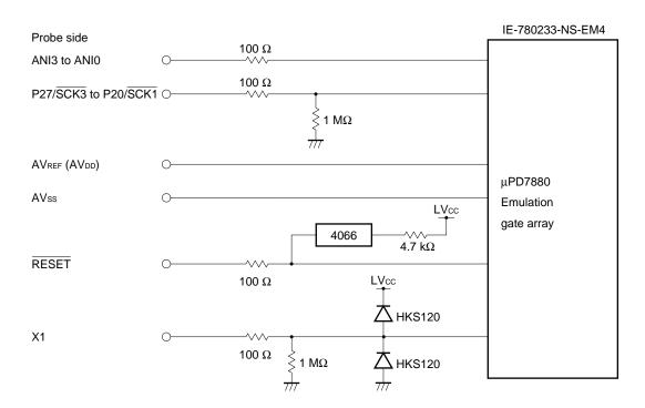
Figure 4-1. Equivalent Circuit of Emulation Circuit 1
