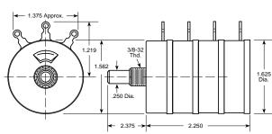
Power Rating: 4 Watts Continuous Ăudio: 15 Watts
