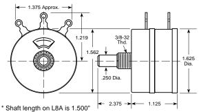
Presents constant impedance to source (Amplifier). Used in audio circuits where output (Speaker) impedance is not critical
