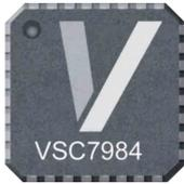
The VSC7984 is a 11.3Gb/s clocked modulator driver for SONET/SDH and 10GbE applications. The device provides selectable data retiming to improve jitter performance and controls for output bias voltage, modulation voltage, and duty cycle. Internal operational amplifiers and on-chip voltage
