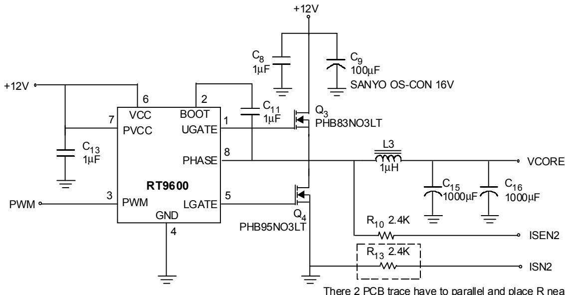
There 2 PCB trace have to parallel and place R near to PWM IC
