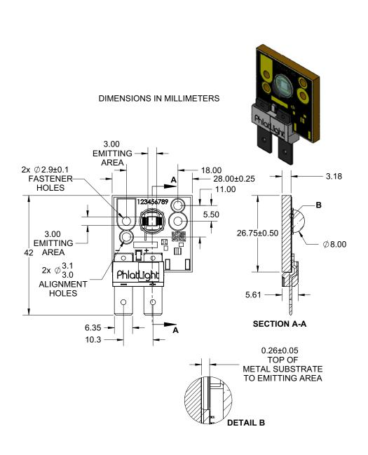
Recommended connector for Anode and Cathode: Panduit Disco Lok™ Series P/N: DNG14-250FL-C For detailed drawing please refer to DWG-001277 document
