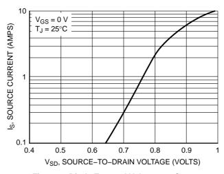
Figure 7. Diode Forward Voltage vs. Current
