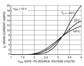
Figure 2. Transfer Characteristics
