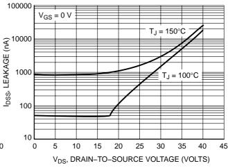
Figure 6. Drain-to-Source Leakage Current vs. Voltage
