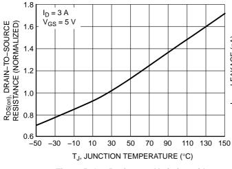
Figure 5. On–Resistance Variation with Temperature
