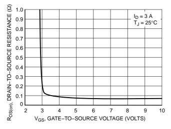
Figure 3. On-Resistance vs. Gate-to-Source Voltage
