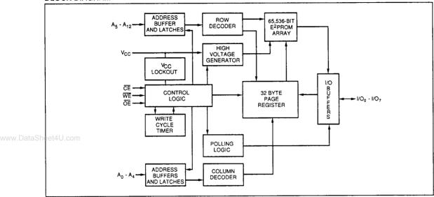
The automatic page write feature allows the system to program up to 32 bytes during a single nonvolatile write cycle, providing an effective write speed of at most 312ms/byte. The entire 8K byte memory may be programmed in a maximum of 2.6 seconds when the page write mode is employed.
