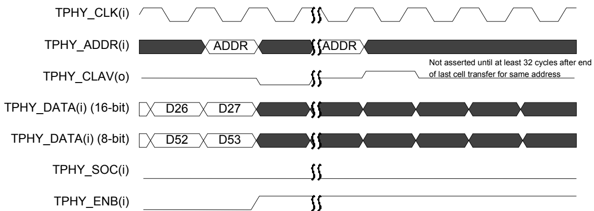
Figure 108 SNK_INTF End-of-Transfer Utopia 2 (Multi-Address PHY Mode)
