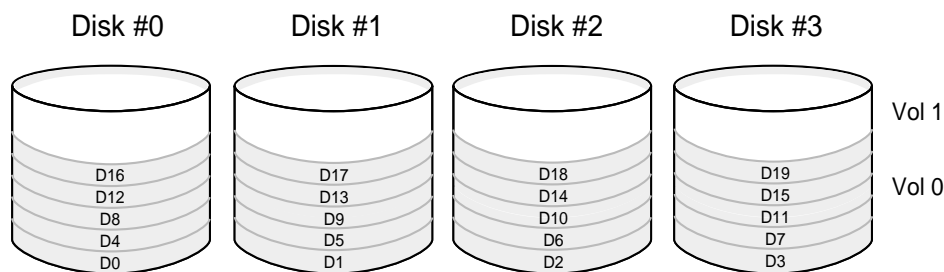
Figure 5-2. Stripes and Strips in a RAID Volume
