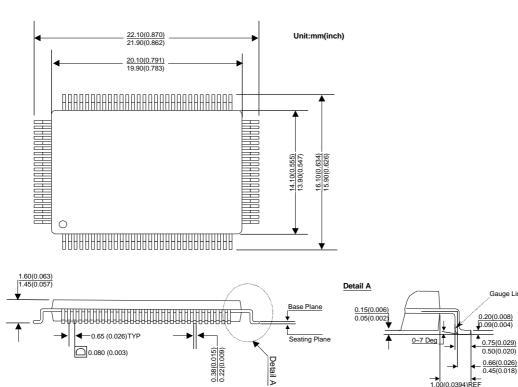
All dimension in mm (inches). Notation is  $\frac{\text{MAX}}{\text{MIN}}$  or typical.
