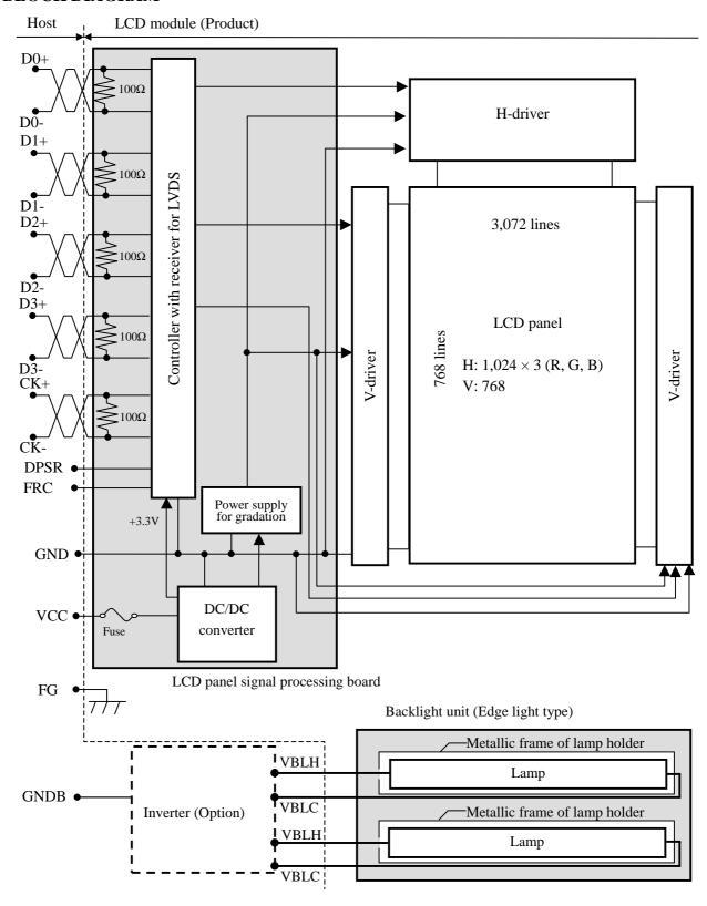
Note1: GND (Signal ground), FG (Frame ground) and GNDB (Backlight inverter ground) should be connected together in customer equipment.
