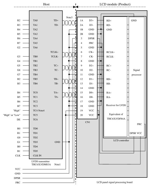
Note1: Recommended transmitter THC63LVDM83A (THine Electronics Inc.).
