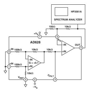
Test Circuit 3. Noise Tests
