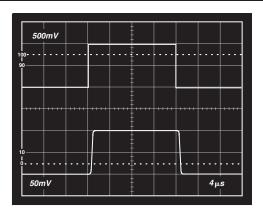
TPC 16. Small Signal Pulse Response,  $R_L = 2 \text{ k}\Omega$ ,  $C_L = 0 \text{ pF}$ , Top: Input, Bottom: Output
