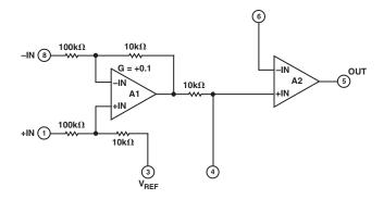
Figure 3. Simplified Schematic
