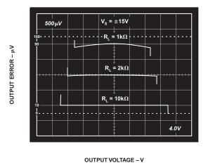
TPC 12. Normalized Gain Error vs.  $V_{OUT}$ ,  $V_S = \pm 15 V$
