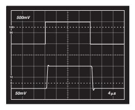
TPC 17. Small Signal Pulse Response,  $R_L = 2 \text{ k}\Omega$ ,  $C_L = 1000 \text{ pF}$ , Top: Input, Bottom: Output
