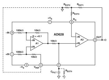
Figure 4. Circuit Connections
