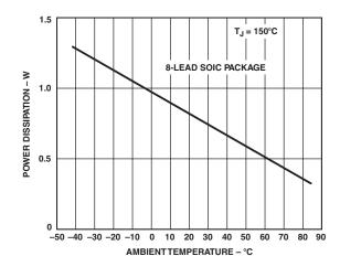
Figure 2. Maximum Power Dissipation vs. Temperature
