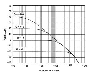
TPC 8. Small Signal Frequency Response,  $V_{OUT1} = 200 \text{ mV p-p}, G = +0.1, +1, +10, \text{ and } +100$
