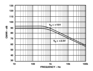
Figure 1. CMRR vs. Frequency of the AD628
