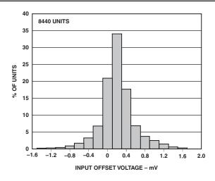
TPC 1. Typical Distribution of Input Offset Voltage,  $V_{\rm S} = \pm 15$  V, SOIC Package
