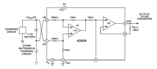
Figure 7. A Battery Voltage Monitor
