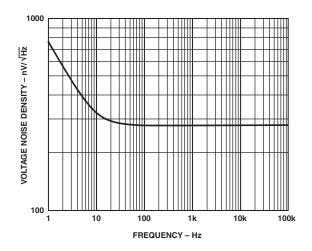
TPC 6. Voltage Noise Spectral Density, RTI,  $V_S = \pm 2.5 V$
