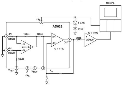
Test Circuit 2. PSRR vs. Frequency
