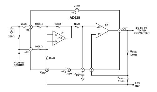
Figure 6. Level Shifter for 4-20 mA Current Loop
