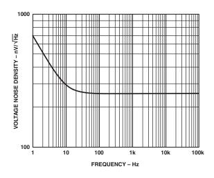
TPC 5. Voltage Noise Spectral Density, RTI,  $V_S = \pm 15 V$
