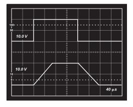
TPC 18. Large Signal Pulse Response,  $R_L = 2 \text{ k}\Omega$ ,  $C_L = 1000 \text{ pF}$ , Top: Input, Bottom: Output
