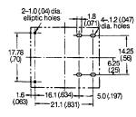
Note: A tolerance of  $\pm 0.10$  mm (0.004 in) applies to all dimensions.
