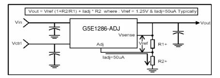
The G5E1286-ADJ keeps a constant 1.25V between the Vsense pin and the Adj pin. By placing a resistor R1 across these two pins and connecting the Vsense and Vout pin together, a constant current flows through R1, adding to the ladj current and into the R2 resistor producing a voltage equal to the (1.25/R1)\*R2+ladj\*R2. This voltage is then added to the 1.25V to set the output voltage. This is summarized in the above equation.
