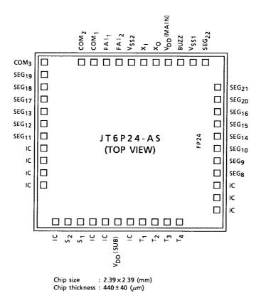
Note 1: Be sure to connect the V<sub>DD</sub> (MAIN).
