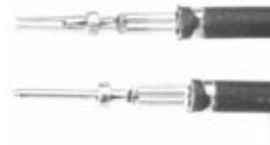
8. Note that there are no unterminated wire strands, and that some strand ends can be seen at the forward edge of the crimp. Also note the insulation is gripped by the smaller secondary crimp. Distortion is at a minimum, both axially and laterally - no sharp edges.
