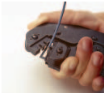
5. Insert the pre-stripped wire into the crimp area of the contact and completely cycle the tool.
