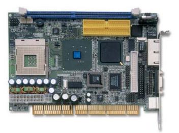
The HS-7238S is an Intel<sup>®</sup> 82845GV/82801DB chipset-based board designed for PCI-ISA Bus PGA 478 Intel<sup>®</sup> Pentium<sup>®</sup> 4 up to 2.8GHz CPU compatibility. The combination of these features makes the HS-7238S an ideal all-in-one industrial single board computer. Additional features include an enhanced I/O with CRT/LVDS Panel, dual LAN, wireless LAN, audio, and USB2.0 port interface.
