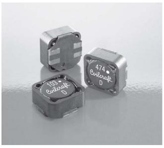
The MSD1260T series of shielded coupled inductors was designed specifically for high temperature applications – up to 125°C. The excellent coupling coefficient  $(k \ge 0.94)$  makes it ideal for use in SEPIC applications. In SEPIC topologies, the required inductance for each winding in a coupled inductor is half the value needed for two separate inductors, allowing selection of a part with lower DCR and higher current handling.
