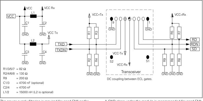
The power supply filtering is required for good EMI performance. Use short tracks from the inductor L1/L2 to the module  $V_{CC}\text{-}Rx/V_{CC}\text{-}Tx.$
