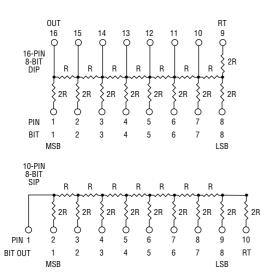
The R/2R Ladder Network is commonly used for Digital to Analog (D/A) conversions and Analog to Digital (A/D) conversion by successive approximations. The bits of the ladder are the points at which input signals are presented to the ladder and the output terminal (OUT) is the point at which the output is
