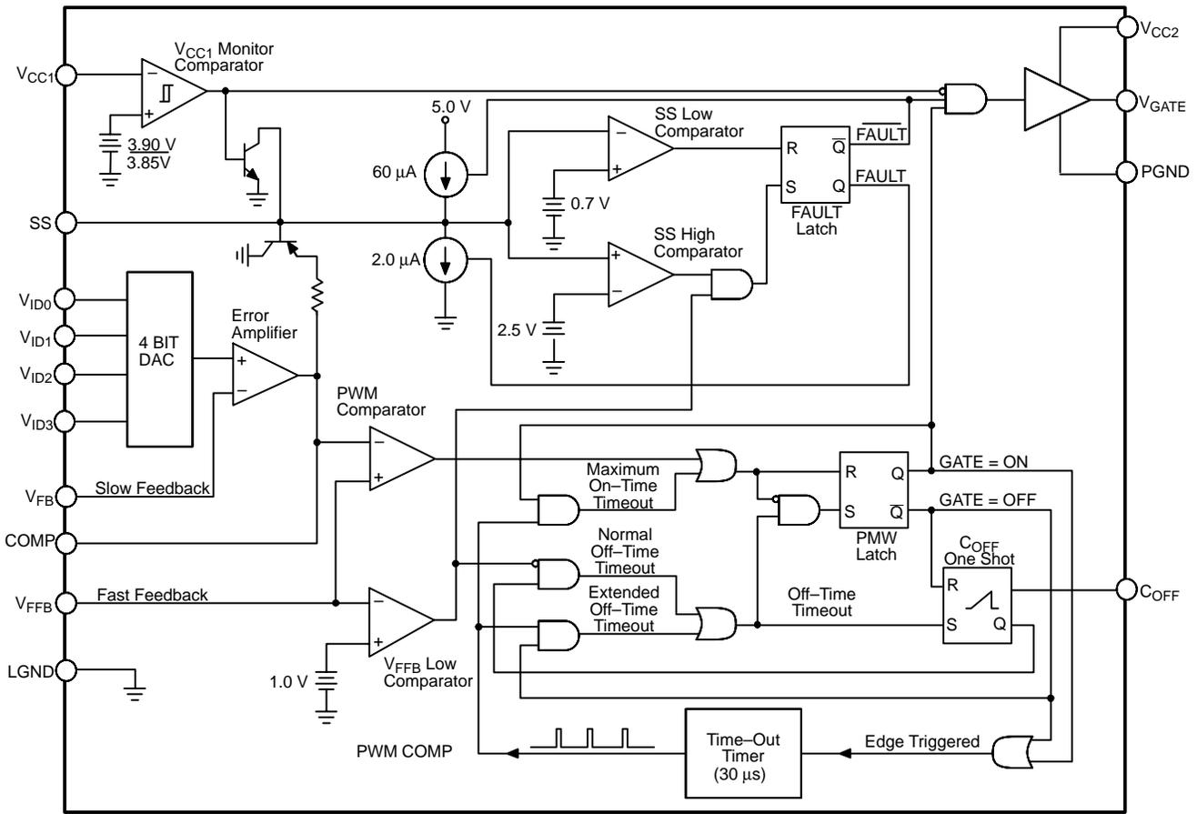
Figure 2. Block Diagram
