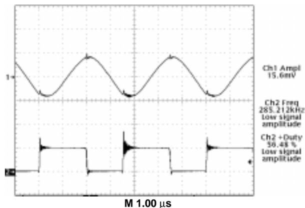
Trace 1– Regulator Output Voltage (10 mV/div.)
