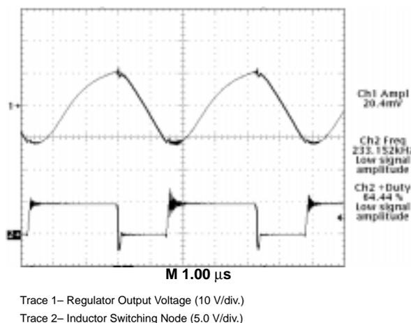
**Figure 8. Peak-to-Peak Ripple on  $V_{OUT} = 2.8$  V,
