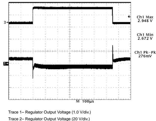
**Figure 9. CS5151 Demonstration Board Response to
