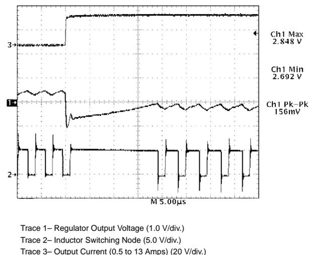
**Figure 10. CS5151 Demonstration Board Response to
