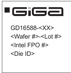
Figure 12. Device marking. Top view. The black square marks location of ball A1.
