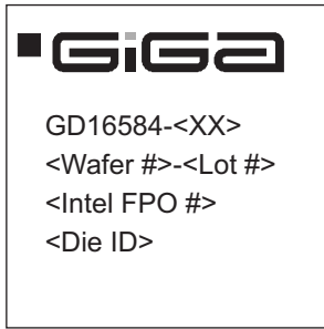
Figure 12. Device marking. Top view. The black square marks location of ball A1.
