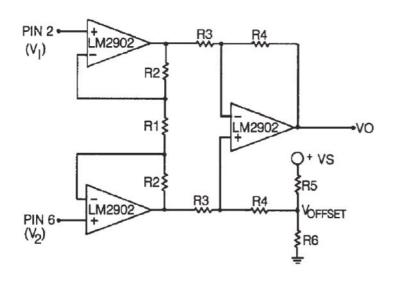
$$V_{O} = \left(\frac{2R_{2} + R_{1}}{R_{1}}\right) \left(\frac{R_{4}}{R_{3}}\right) (V_{2} - V_{1}) + V_{Offset}$$
