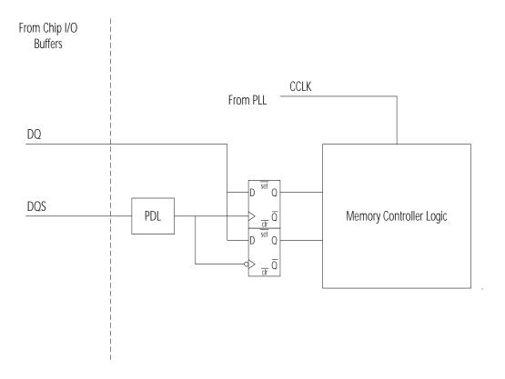
Figure 16. AMD-761™ System Controller DDR Interface Inputs Conceptual Block Diagram
