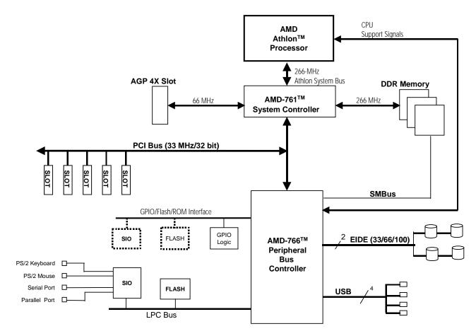
Figure 1. AMD-760™ Chipset System Block Diagram
