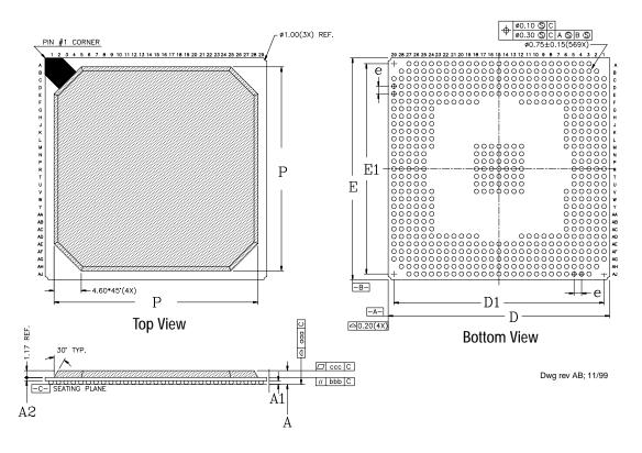
Figure 23. 569-Ball Plastic Ball Grid Array (PBGA) Package
