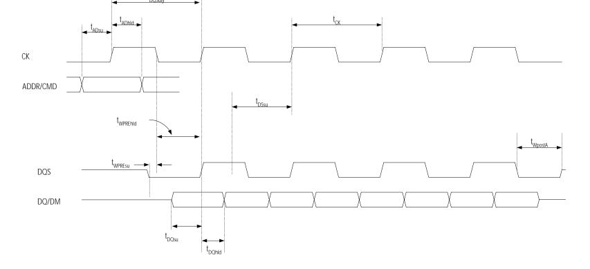
**Note:** Timing parameter symbols defined at controller interface, not at memory device interface.
