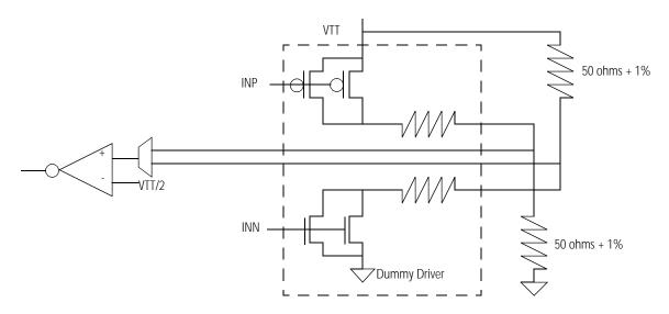
Figure 3. Dummy Load with External Compensation Resistors
