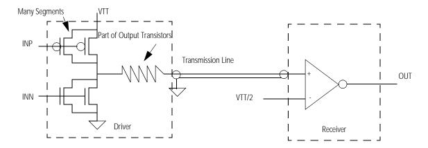
Figure 2. Push-Pull Transmission Line Example
