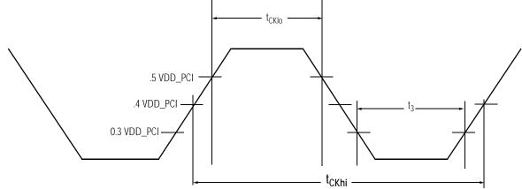
Figure 11. **AGPCLK and PCICLK Waveform**
