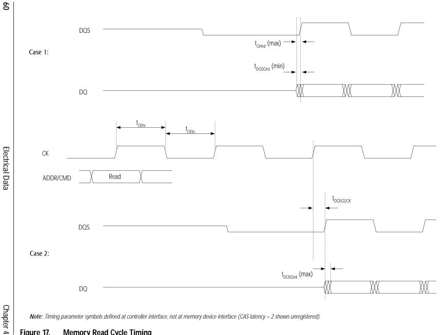
**Note**: Timing parameter symbols defined at controller interface, not at memory device interface (CAS latency = 2 shown unregistered).
