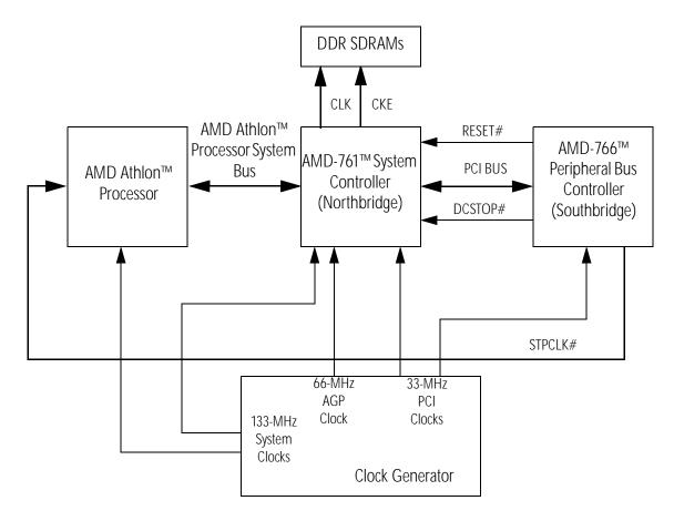
Figure 7. Power Management Signal Connections
