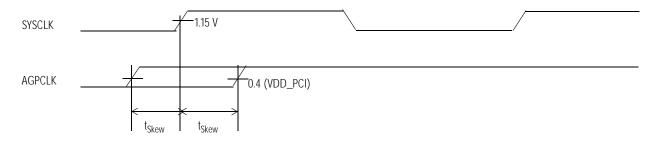
Figure 12. **Clock Skew Requirements**
