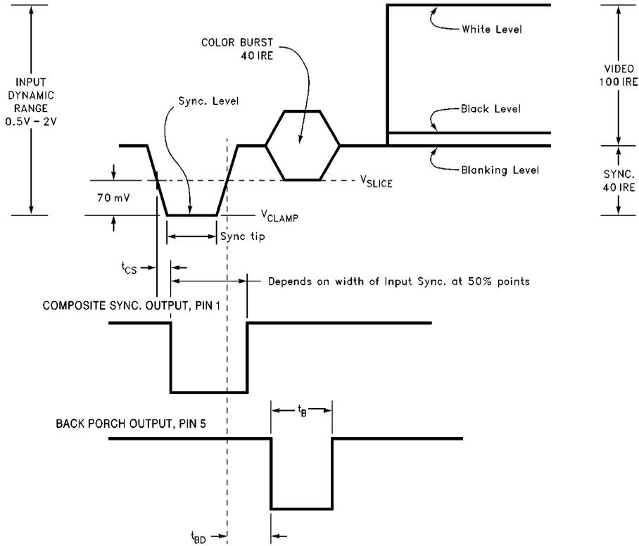
**Figure 4. Standard (NTSC Input) H. Sync Detail**
