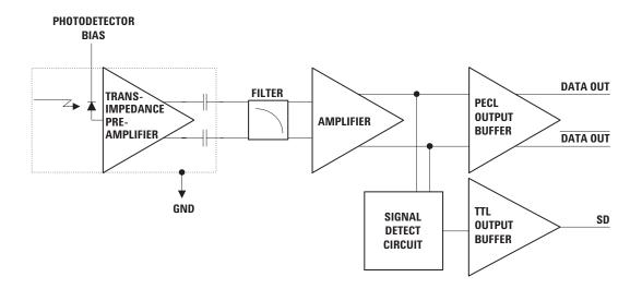
Figure 1 - Receiver Block Diagram
