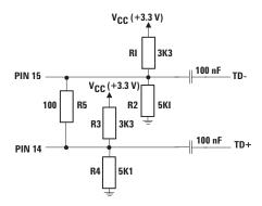
Figure 7b. Low current dc biasing scheme
