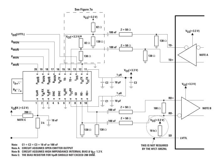
Figure 7 - Recommended Interface Circuit (HFCT-5952TL/TG/ATL/ATG)
