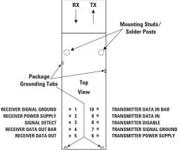
Figure 6 - Pin Out Diagram (Top View)
