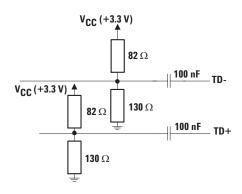
Figure 7a.LVPECL termination and biasing scheme
