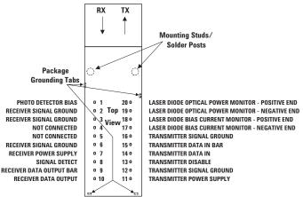
Figure 5 - Pin Out Diagram (Top View)
