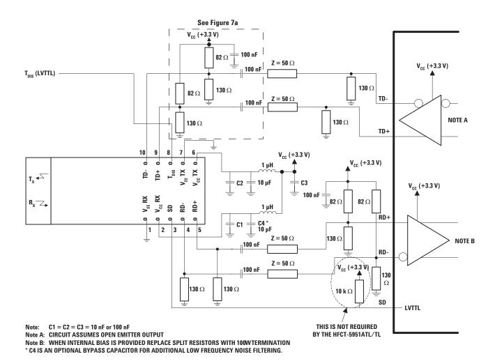
Figure 8 - Recommended Interface Circuit (HFCT-5951TL/TG/ATL/ATG)
