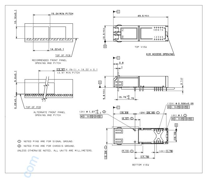
The SFF-PTH-SW/LW-2X5/2X6 is intended to be used on a host card having a thickness of 0.062" to 0.100". The host card footprint with essential keepouts and drill holes is shown in Host Card Footprint (2 X 5 Pin Configuration) on page 18.
