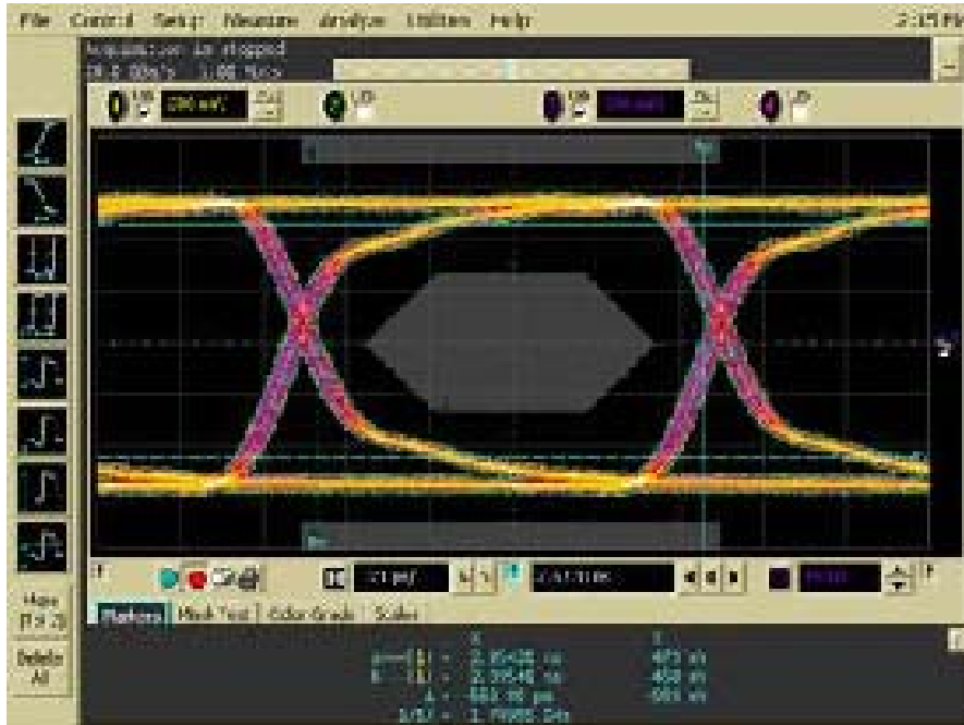
Figure 3: 8bit deep color DVI/HDMI TX eye tested with 2 meter. 30 AWG HDMI cable. Setting: Optimized equalization, 0dB output pre-emphasis and de-emphasis, and Swing 500mV.
