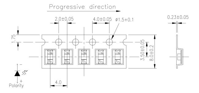
**Note:** Tolerances Unless Dimension  $\pm 0.1$ mm, Unit = mm
