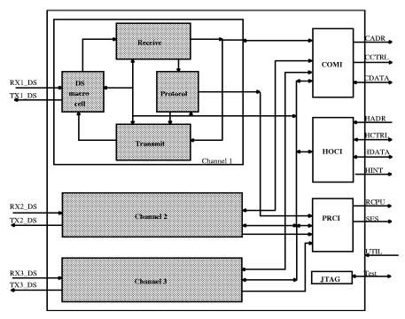
Target applications are heterogeneous multi-processor systems supported by scalable interfaces including the little/ big endian swapping. The TSS901E connects modules with different processors (e.g. 21020F, ERC32, TSC695E and others). Any kind of network topology could be realized through the high speed point-to-point IEEE1355-links (see chapter Applications).
