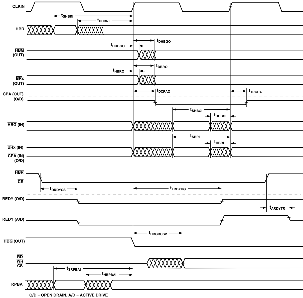
Figure 18. Multiprocessor Bus Request and Host Bus Request
