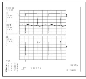
Figure 3 shows the ON and OFF switching traces of the high side MOSFET.
