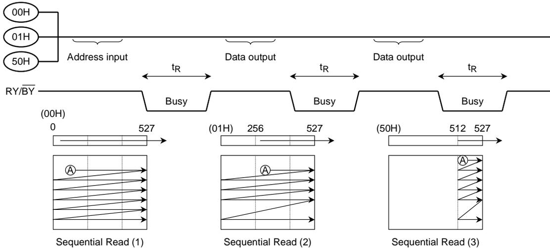
Sequential Read modes (1) and (2) output the contents of addresses 0 to 527 as shown above, while Sequential Read mode (3) outputs the contents of the redundant address locations only.
