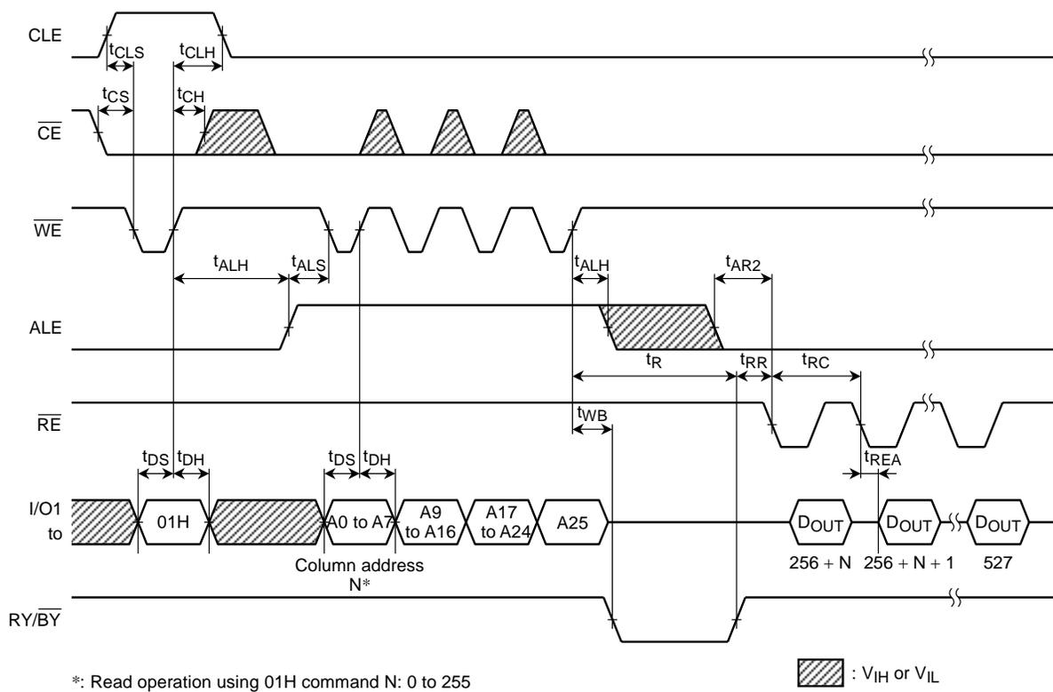
Read Cycle (3) Timing Diagram
