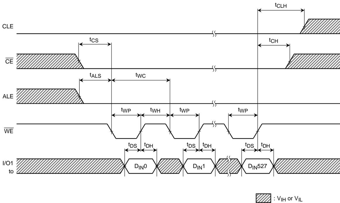
Serial Read Cycle Timing Diagram
