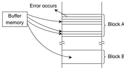
When an error happens in Block A, try to reprogram the data into another Block (Block B) by loading from an external buffer. Then, prevent further system accesses to Block A (by creating a bad block table or by using an another appropriate scheme).
