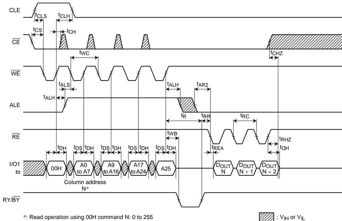
\*: Read operation using 00H command N: 0 to 255
