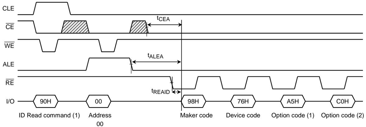
For the specifications of the access times  $t_{READ}$ ,  $t_{CR}$  and  $t_{AR1}$  refer to the AC Characteristics.
