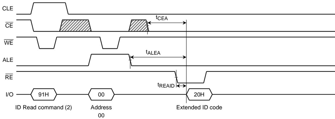
For the specifications of the access times t<sub>READ</sub>, t<sub>CEA</sub> and t<sub>ALEA</sub> refer to the AC Characteristics.
