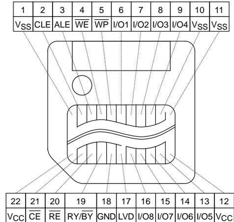
Figure 1. Pinout
