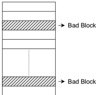
Referring to the Block status area in the redundant area allows the system to detect bad blocks in the accordance with the physical data format issued by the SSFDC Forum. Detect the bad blocks by checking the Block Status Area at the system power-on, and do not access the bad blocks in the following routine.
