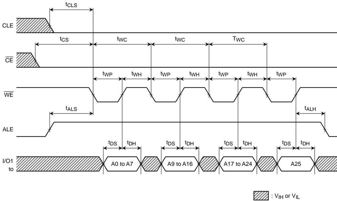
Data Input Cycle Timing Diagram
