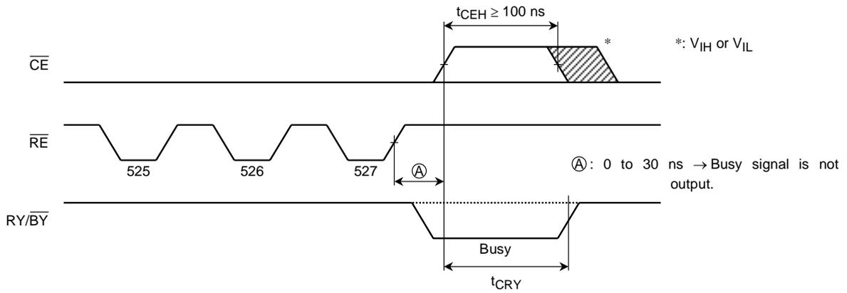
**PROGRAMMING AND ERASING CHARACTERISTICS (Ta = 0° to 55°C, VCC = 3.3 V ± 0.3 V)**
