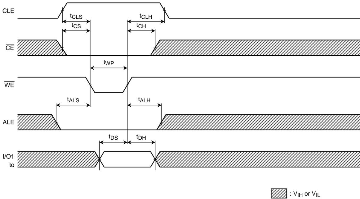
Address Input Cycle Timing Diagram
