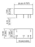
Note: Unit:mm(inch) Pin section:0.50\*0.30mm(0.020\*0.012inch) Pin tolerances:±0.10mm(±0.004inch) General tolerances:±0.25mm (±0.010inch)
