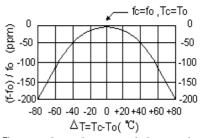
The curve shown above accounts for resonator contribution only and does not include LC component temperature characteristics.
