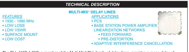
The DLL-115R-1.96G, a member of the Multi-Mix<sup>®</sup> DLL family of delay lines, provides a mean delay of 11.45 nS in the PCS band and features low insertion loss and low VSWR. The DLL-115R-1.96G exhibits excellent phase linearity and amplitude flatness over the 1930 - 1990 MHz frequency range. The Multi-Mix<sup>®</sup> DLL-115R-1.96G is intended for use in power amplifier linearization networks such as feedforward and predistortion.
