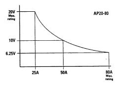
These compact autoranging bench or systems power supplies use a switch-mode topology to provide a wide range of adjustable voltage and current combinations within a 3 kilowatt power envelope.
