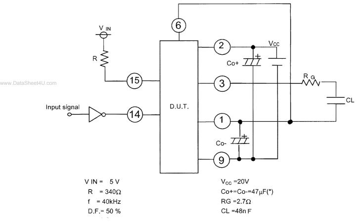
(\*) Please mount the capacitor for the voltage amends as much as possible near hybrid IC.
