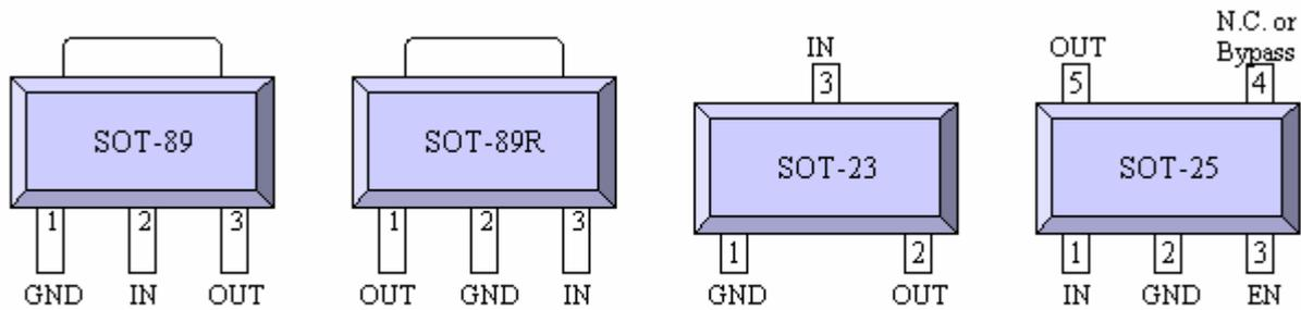
Figure 2 : pin configuration
