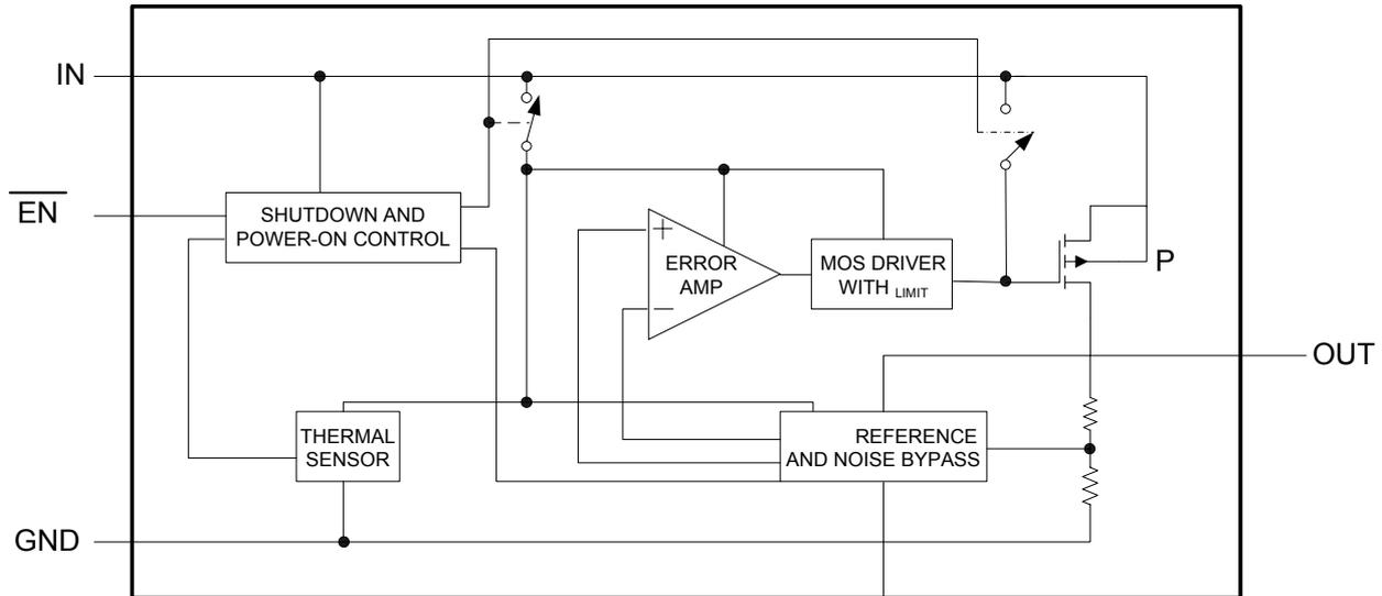
Figure 3. Block Diagram
