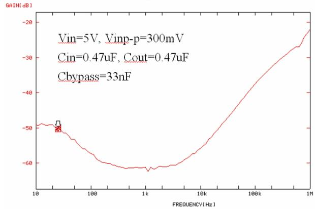
**PSRR vs Frequency (Load=100mA)**
