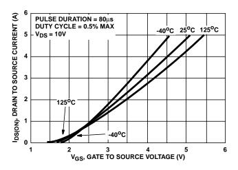
FIGURE 5. TRANSFER CHARACTERISTICS
