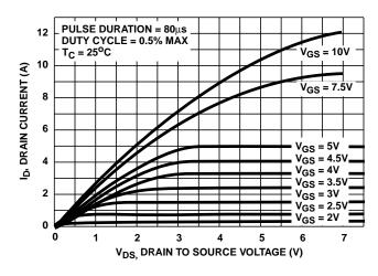
FIGURE 4. SATURATION CHARACTERISTICS
