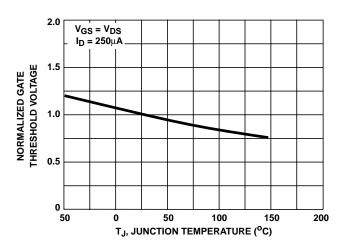
FIGURE 8. NORMALIZED GATE THRESHOLD VOLTAGE vs JUNCTION TEMPERATURE
