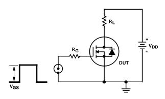
FIGURE 11. SWITCHING TIME TEST CIRCUIT
