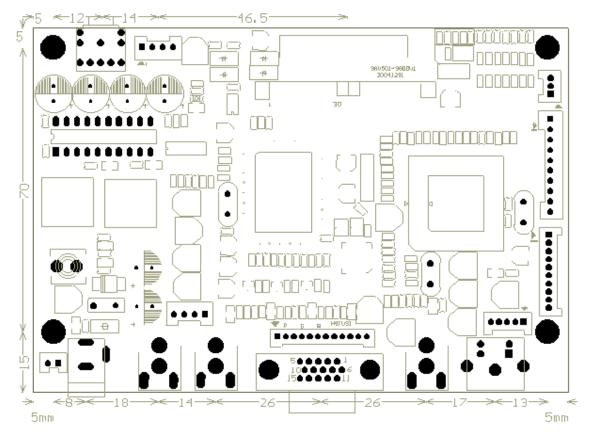
Outline: 132.0\*90.0\*17.1mm Top Layer High (Max): 13.0 mm Bottom Layer High (Max): 2.5 mm Board Thickness: 1.6mm Screws: D3.0mm\*4
