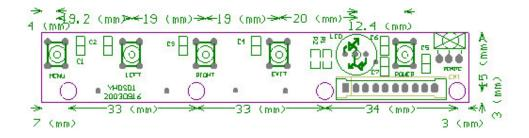
Outline: 110.0\*18.0\*7.1mm Top layer High (Max): 5.5 mm Board Thickness: 1.6 mm Screw: D3.0mm
