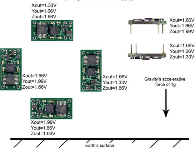
The voltage outputs on the DE-ACCM3D correspond to acceleration being experienced in the X, Y and Z directions. The output is ratiometric, so the output sensitivity (in mV/g) will depend on the supply voltage.
