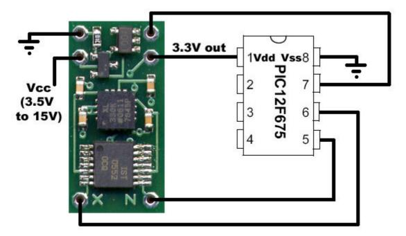
Additional capacitance across the microcontroller's power pins may be necessary, depending on your particular setup.
