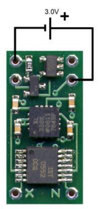
This would be useful for e.g. an application powered directly by 2 AA batteries or a lithium coin battery. The minimum operating voltage when using bypass mode is 2.0V and **the absolute maximum voltage that can be applied when bypassing the regulator is 3.6V.**
