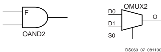
Figure 7: AND and MUX Symbols in Spartan-XL IOB
