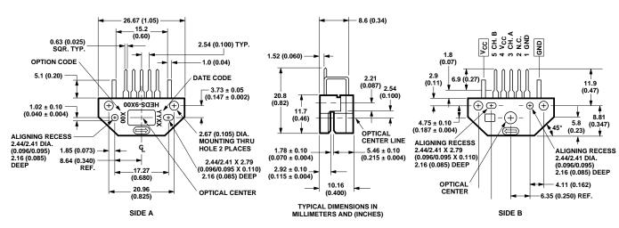
For the HEDS-9100, standard resolutions between 96 CPR and 512 CPR are available for use with a HEDS-5120 codewheel or equivalent.
