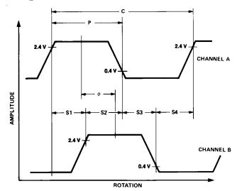
by the pattern of spaces and bars on the codewheel. The photodiodes which detect these interruptions are arranged in a pattern that corresponds to the radius and design of the odewheel. These detectors are also spaced such that a light period on one pair of detectors corresponds to a dark period on the adjacent pair of detectors. The photodiode
